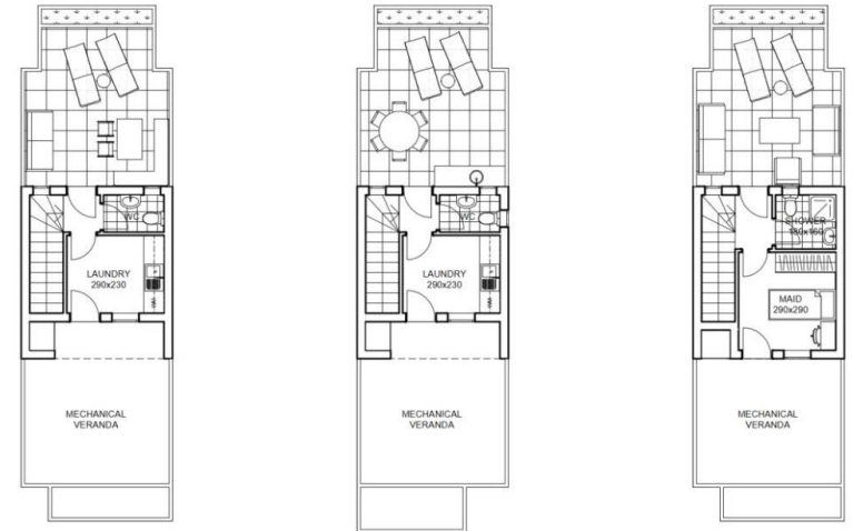
TYPE A.1 TWO BEDROOM HOUSE parking in front INTERNAL COVERED AREA 17.60M 2 EXT. COVERED AREA 4.84M 2 EXT. UNCOVERED AREA 36.54M 2
