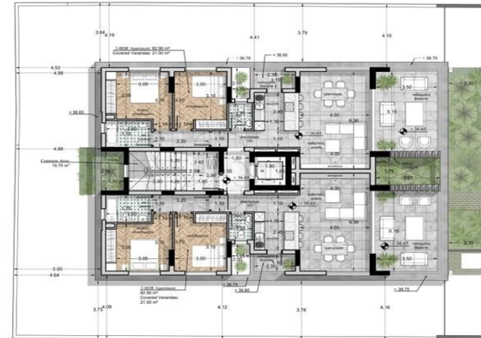
Layout approach 1st Floor / 2nd Floor / 3rd Floor / 4th Floor: 19.70m 2 (common area) + 82.90m 2 (2-BDR) + 82.90m 2 (2-BDR) = 185.50 m 2 Covered Verandas: 21.50m 2 (2-BDR) + 21.50m 2 (2-BDR) = 43.00 m 2 (23.18%)
