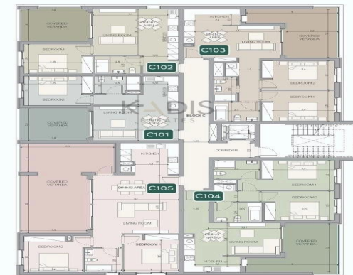
BLOCK C 1ST FLOOR PLAN 1:100
