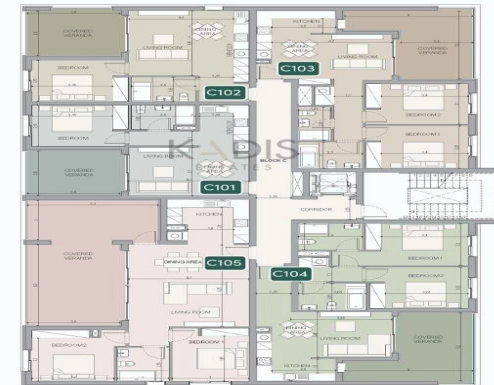
BLOCK C 1ST FLOOR PLAN 1:100
