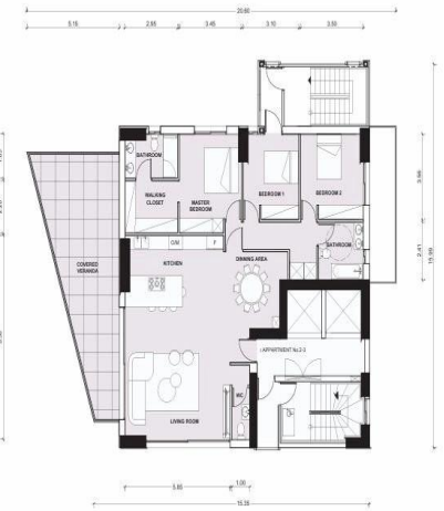
2nd-3rd FLOOR PLAN SCALE 1:100
