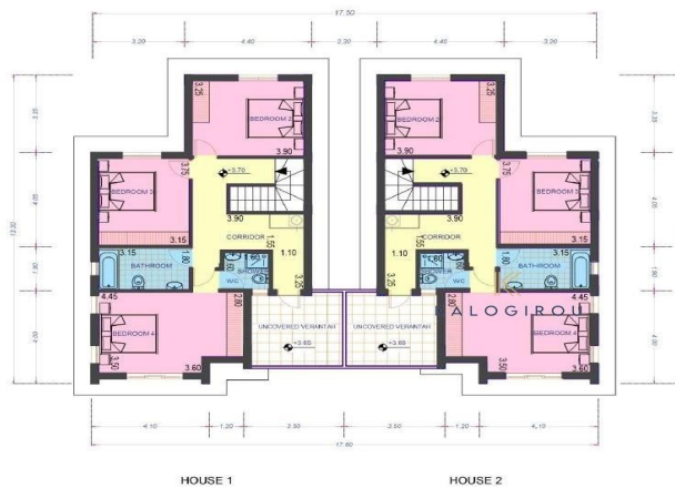
FIRST FLOOR PLAN SCALE 1-100
