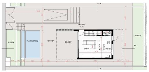
HOUSE TYPE C- HOUSES 17-22 TWO STOREY HOUSE WITH ROOF GARDEN GROUND FLOOR PLAN
