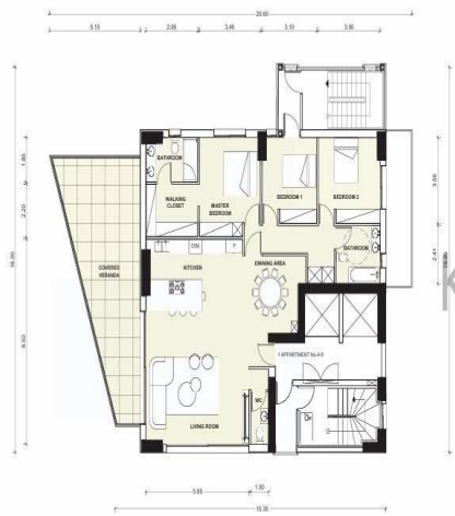
4th-9th FLOOR PLAN SCALE 1:100
