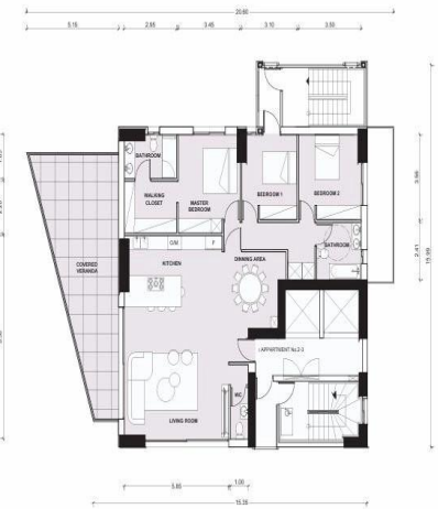
2nd-3rd FLOOR PLAN SCALE 1/100
