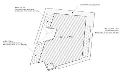
first floor build density = 6B = 107m<sup>c</sup>
