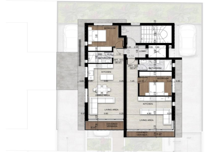
1. FIRST FLOOR PLAN
