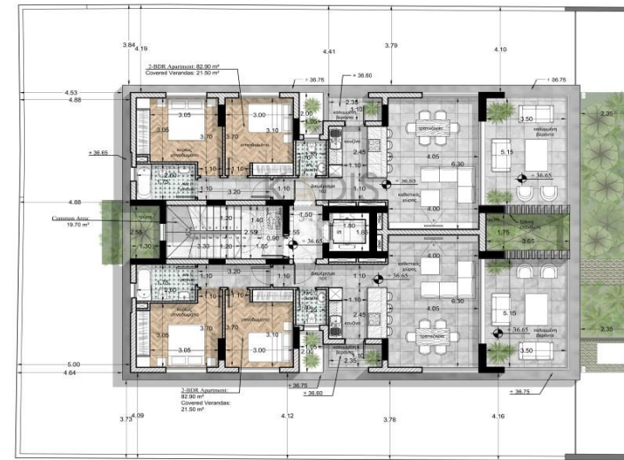
Layout approach 1st Floor / 2nd Floor / 3rd Floor / 4th Floor: 19.70m 2 (common area) + 82.90m 2 (2-BDR) + 82.90m 2 (2-BDR) = 185.50 m 2 Covered Verandas: 21.50m 2 (2-BDR) + 21.50m 2 (2-BDR) = 43.00 m 2 (23.18%)
